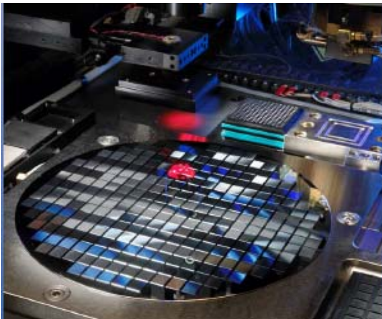
Die to Wafer alignment and placement
