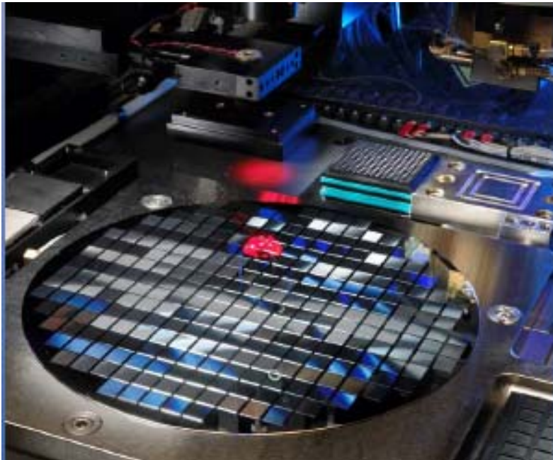
1 Mpixel, 8 um pitch die being mounted to 200 mm "ROIC" wafer
