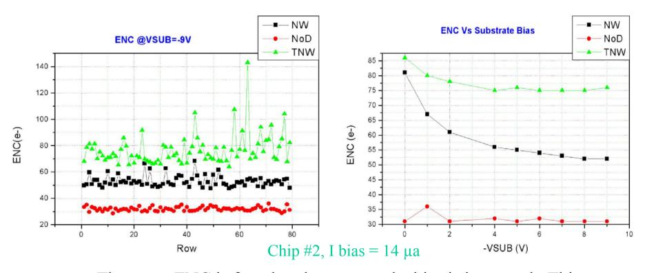
The mean ENC is found to decrease as the bias is increased. This believed to be due to the decreasing value of the diode capacitance.
