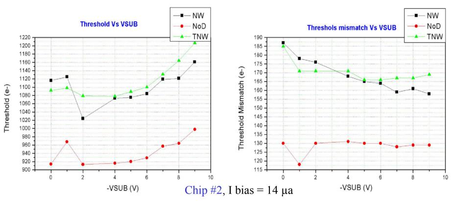
Beginning at about -5 volts, the average threshold was found to increase for all 3 types of circuits. This is thought to be due to the kill and inject logic failing to pass all hits. Threshold mismatch for diode circuits is found to get smaller with increasing Vsub due to increase in gain as diode capacitance gets smaller.
