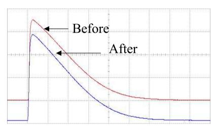
Output of 2<sup>nd</sup> stage (after buffer) before and after irradiation for input charge of 10 ke<sup>-</sup>.
