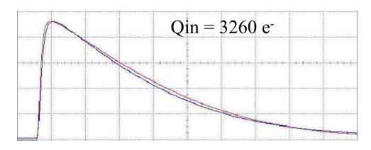
Buffered output of second stage before and after 33 Mrads. Exact same bias settings used for both measurements. Observed 3 mv offset change, 5% change in rise and fall times.
