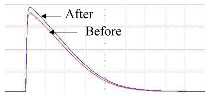
Output of 2<sup>nd</sup> stage before and after irradiation, with the after signal shifted (on the scope) to correct for 100 mV offset. The same shift can be made by changing Vfb2 which is programmable.
