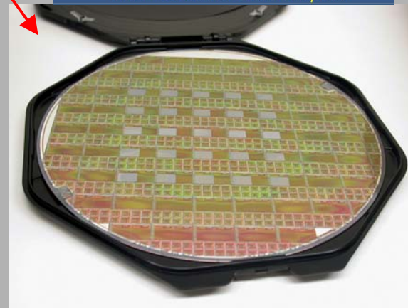
Sensors thinned to 100 μm after chip to wafer bonding
