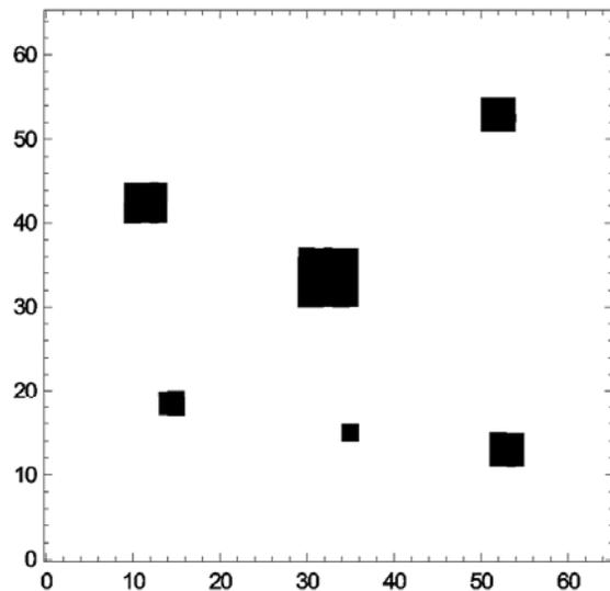
Hit pattern injected into pixel array
