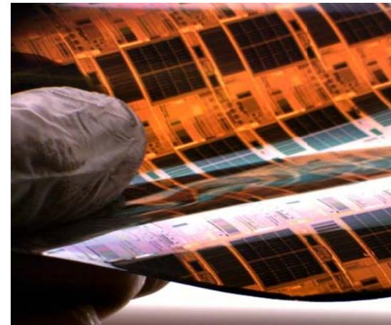
6 inch SOI wafer thinned to 6 μm and mounted to 3 mil kapton for support at MIT LL
