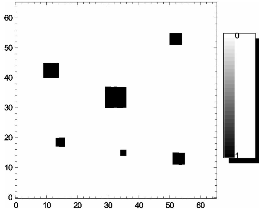
**Preselected pattern** of pixels for the injection of signal to the front-end amplifiers; pattern shifted into the matrix, then positive voltage step applied across the injection capacitance; threshold levels for the discriminator adjusted according to the amplitude of the injected signal
