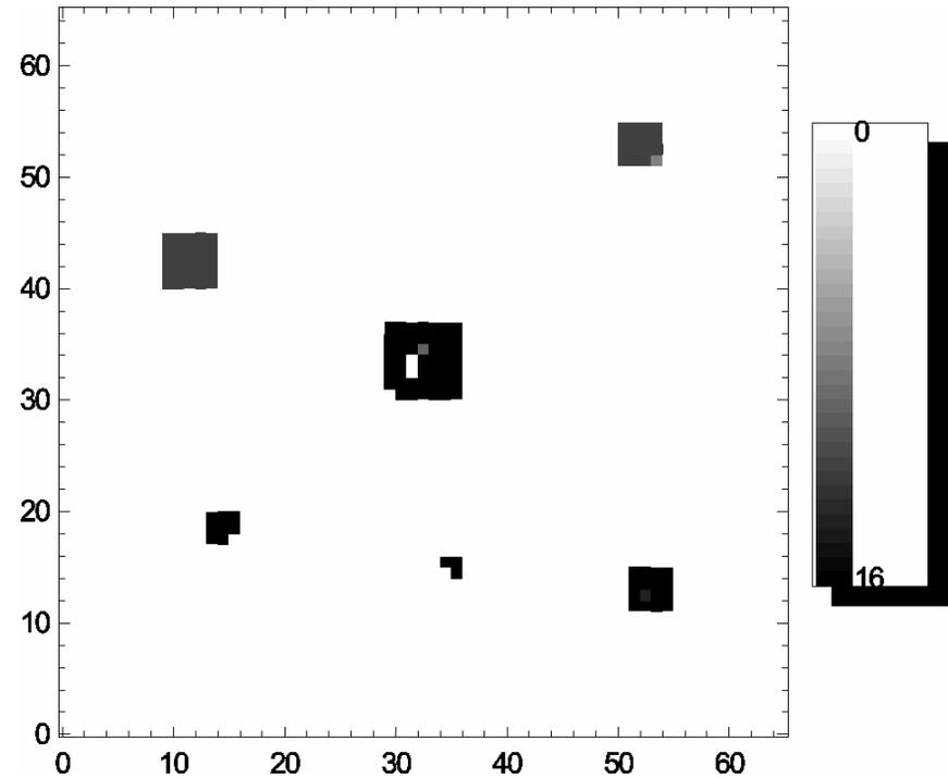
Pattern of pixels from the preselected injection pattern that after injection of tests charge reported as hit (grey level represents number of repetition - 8 times injection)
