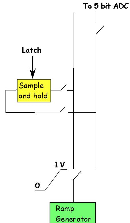
Ramp operates at low speed for low power.
