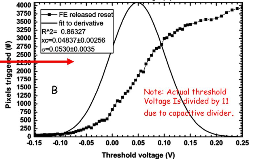
The threshold shift between A and B and the increase in dispersion is thought to be due to internal coupling problems.
