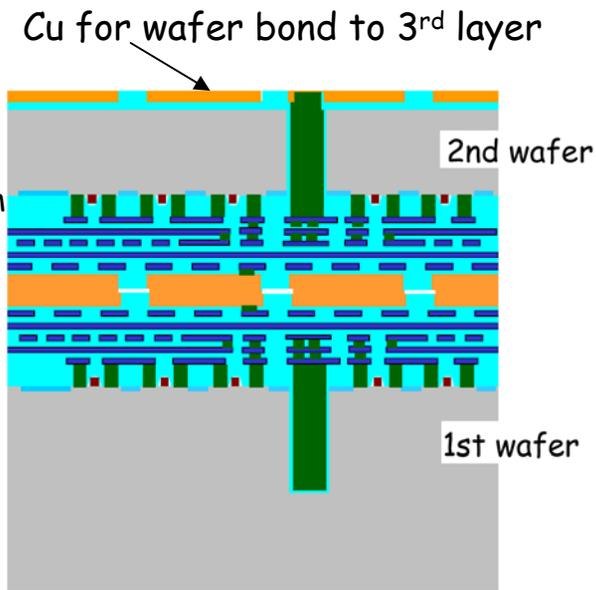
Thin second wafer to about 12um to expose super via.
