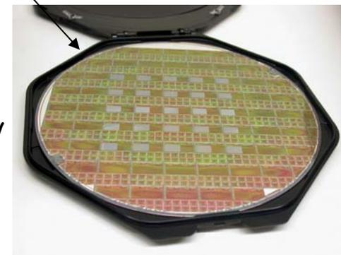
Sensors thinned to 100 um after chip to wafer bonding
