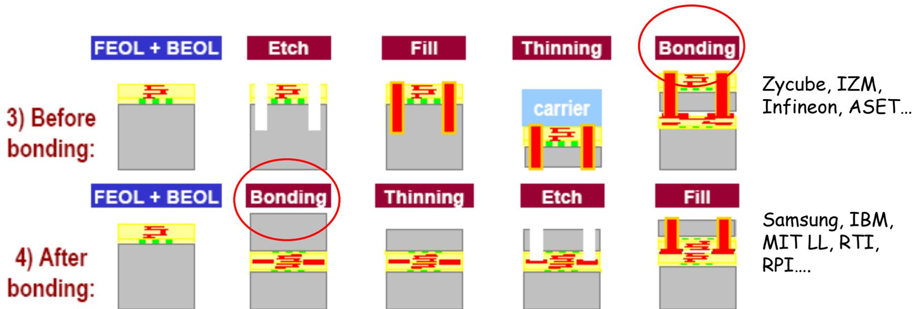
Notes: Vias take space away from all metal layers. The assembly process is streamlined if you don't use a carrier wafer.
