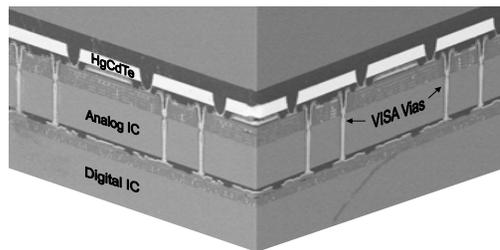
256 x 256 Infrared Pixel Array<sup>4</sup>
