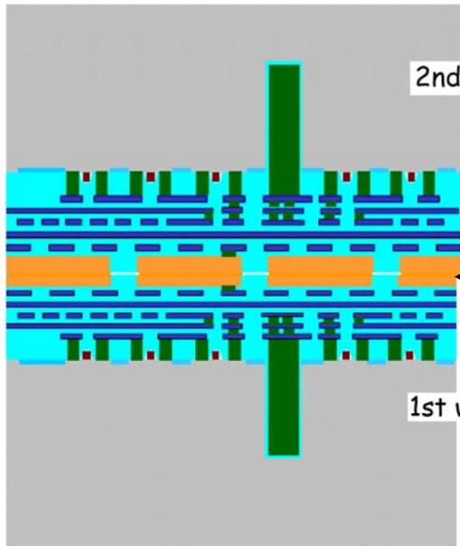
Flip 2<sup>nd</sup> wafer on top of first wafer.
