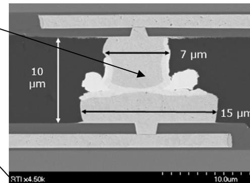
25 Pixel sensors bonded to BTEV ROIC wafer
