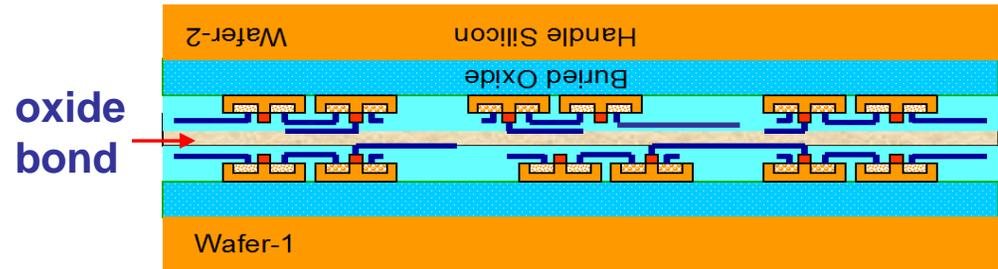
**Step 3: Remove handle silicon from wafer 2, etch 3D Vias, deposit and CMP tungsten**
