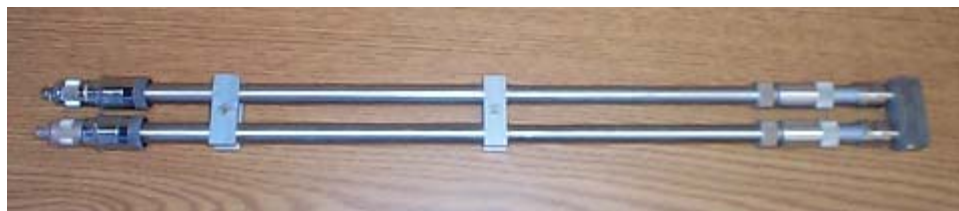
Constant impedance trombone picosecond line
