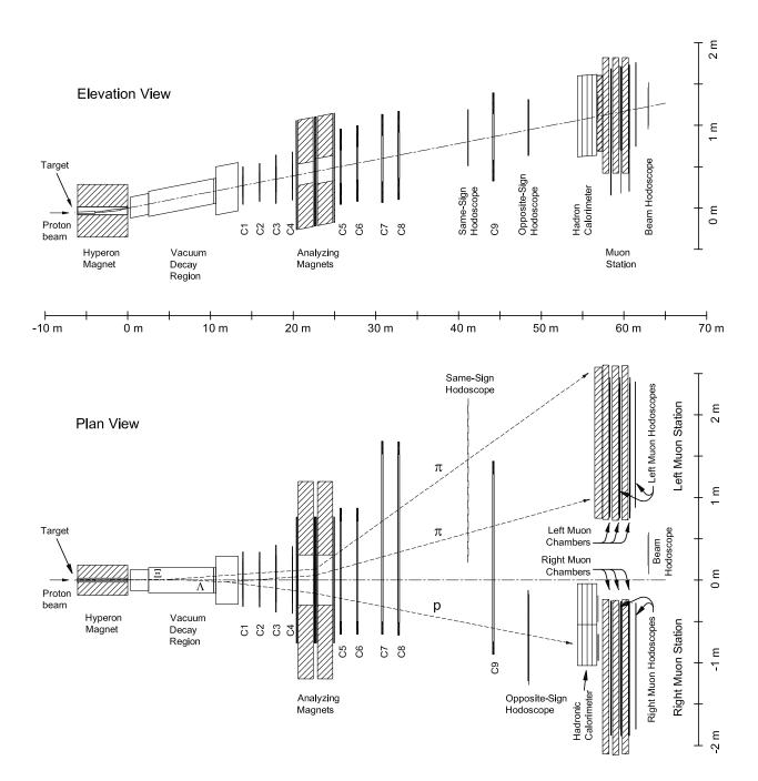
Elevation and plan views of the HyperCP spectrometer. The 1999 configuration is shown. Superimposed on the plan view are the charged tracks of a  $\Xi \to \Lambda \pi \to p\pi\pi$  decay. For clarity, enclosures, support structures, and helium bags are not shown. Transverse dimensions have been exaggerated by a factor of ten.
